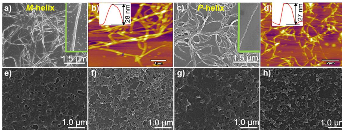
Fig. 2 SEM and AFM images of supramolecular structures of (a and b)  $\text{Ag}^+-\text{L-1}$  formed in THF, and (c–d)  $\text{Ag}^+-\text{D-1}$  in (c and d) THF, (e) EtOH, (f) MeOH, (g)  $\text{CH}_3\text{CN}$  and (h)  $\text{H}_2\text{O}$ . The insets in (a) and (c) show, respectively, two types of polymeric structures, namely the *M*-helix of  $\text{Ag}^+-\text{L-1}$  and *P*-helix of  $\text{Ag}^+-\text{D-1}$ .  $[\text{Ag}^+-\text{L-1}] = [\text{Ag}^+-\text{D-1}] = 25 \mu\text{M}$ .
