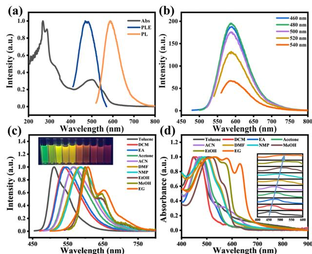
**Fig. 2** (a) UV-vis absorption (black), PL (orange), and PLE (blue) spectra of CDs in DMF. (b) The PL spectra of CDs at different excitation wavelengths in DMF. (c) Normalized fluorescence spectra of O-CDs in different solvents. The inset shows normalized photographs of O-CDs under UV light. (d) Normalized absorption spectra of O-CDs in different solvents. The inset shows the red-shift trend of the absorption peaks between 400 and 600 nm.
