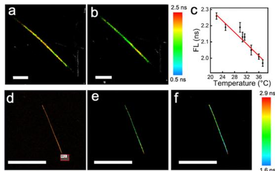
**Fig. 1** The FLIM images of the NWFLT at 25.0 °C (a) and 36.0 °C (b), the FL of the single NWFLT vs. temperature (c). (d) The fluorescence image of the single NWFLT, the red rectangular area (S1:1) was stimulated with a 561 nm laser. The FLIM images of the NWFLT before (e) and after (f) stimulation with a 561 nm laser for 10 min. The scale bars in (a) and (b) are 10  $\mu\text{m}$ , and in (d), (e) and (f) are 60  $\mu\text{m}$ .
