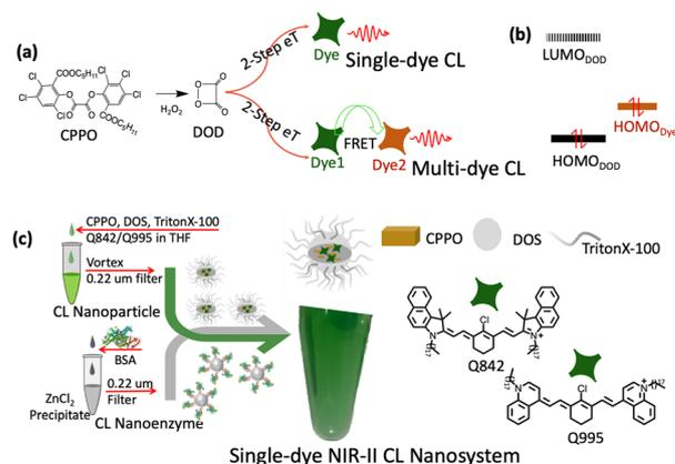
**Scheme 1** (a) The CL mechanism of single-dye CL and multi-dye CL. (b) The frontier orbitals of DOD and the dye. (c) The preparation of the single-dye NIR-II CL nanosystem of cyanine dye Q995 and Q842.
