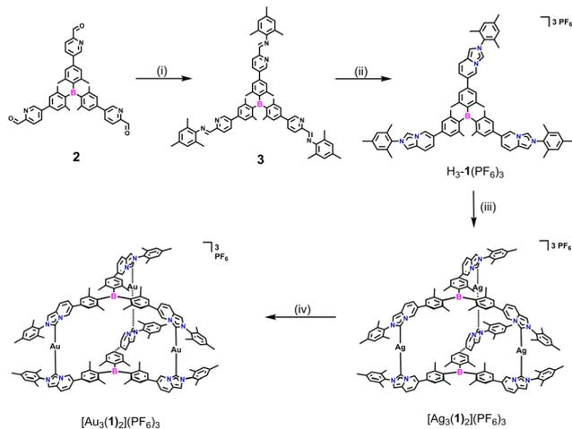
**Scheme 1** Synthesis of the triarylborane-bridged NHC precursor  $H_3-1(PF_6)_3$  and trinuclear hexacarbene complexes. (i) 2,4,6-Trimethylaniline,  $CH_3COOH$ ,  $CHCl_3/EtOH$ , reflux; (ii) (a) paraformaldehyde,  $HCl$ ,  $25\text{ }^\circ C$ ; (b)  $NH_4PF_6$ ,  $MeOH$ ,  $25\text{ }^\circ C$ , yield 51%; (iii)  $Ag_2O$ ,  $CH_3CN$ ,  $55\text{ }^\circ C$ , yield 96%; (iv)  $AuCl(THT)$ ,  $CH_3CN$ ,  $25\text{ }^\circ C$ , yield 83%.
