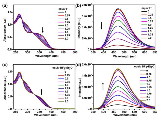
**Fig. 5** (a) The UV-vis absorption and (b) fluorescence emission spectra of  $[Au_3(1)_2](PF_6)_3$  with TBAF (tetrabutylammonium fluoride). (c) The UV-vis absorption and (d) fluorescence emission spectra of  $[Au_3(1)_2](PF_6)_3$  with  $BF_3 \cdot Et_2O$  in the presence of 2 equivalents of TBAF ( $CH_3CN$ ,  $\lambda_{ex} = 330$  nm,  $c = 10^{-5}$  M, and  $T = 298$  K).
