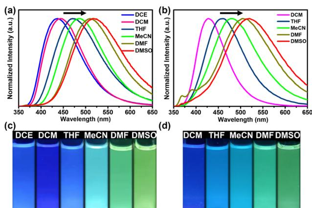
**Fig. 4** The normalized fluorescence emission spectra of (a)  $[Ag_3(1)_2](PF_6)_3$  and (b)  $[Au_3(1)_2](PF_6)_3$  in various solvents ( $\lambda_{ex} = 330$  nm,  $c = 10^{-5}$  M, and  $T = 298$  K). Photographs of (c)  $[Ag_3(1)_2](PF_6)_3$  and (d)  $[Au_3(1)_2](PF_6)_3$  in various solvents under UV light.
