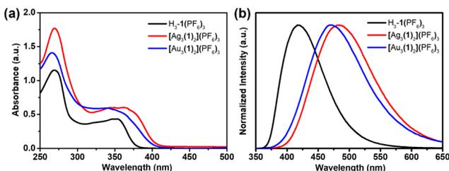
**Fig. 3** (a) The UV-vis absorption and (b) normalized emission spectra of  $H_3-1(PF_6)_3$ ,  $[Ag_3(1)_2](PF_6)_3$ , and  $[Au_3(1)_2](PF_6)_3$  in acetonitrile solution ( $\lambda_{ex} = 330$  nm,  $c = 10^{-5}$  M, and  $T = 298$  K).
