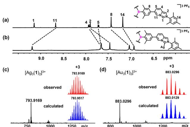
**Fig. 1** Sections of the  $^1H$  NMR spectra (600 MHz,  $CD_3CN$ ) of (a)  $H_3-1(PF_6)_3$  and (b)  $[Ag_3(1)_2](PF_6)_3$ . The HR-ESI mass spectra of (c)  $[Ag_3(1)_2](PF_6)_3$  and (d)  $[Au_3(1)_2](PF_6)_3$  (experimental in red, calculated in blue).
