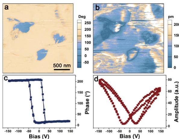
Fig. 3 Vertical PFM phase (a) and amplitude (b) images on the crystal surface of MPSnI<sub>3</sub> at 288 K. Vertical PFM phase (c) and amplitude (d) signals *versus* the tip bias at a selected location.
