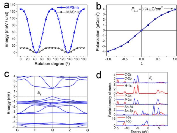
Fig. 4 (a) Rotational energy barrier of MP and MA cations in the inorganic SnI<sub>3</sub><sup>−</sup> framework. (b) Evolution path of polarization with structural distortion of MPSnI<sub>3</sub>. (c) The energy-band structure of a MPSnI<sub>3</sub> crystal shows a direct bandgap of 1.58 eV. (d) The partial density of states (PDOS) of a MPSnI<sub>3</sub> crystal.
