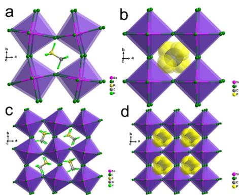
**Fig. 1** Basic structures for  $\text{MPSnI}_3$  at (a) 273 K, and (b) 313 K, respectively. The P atom and C atom of the  $\text{MP}^+$  cation are disordered over the two possible positions. Only one distribution is illustrated for clarity. Packing view of the structures for  $\text{MPSnI}_3$  at (c) 273 K, and (d) 313 K, respectively. H atoms of the organic cations in HPP were not modeled because of total disorder, and thus not shown in (b) or (d).
