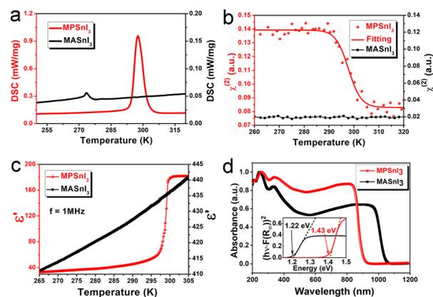
**Fig. 2** (a) DSC measurements revealed a structural phase transition at around  $T_c = 298$  K ( $\text{MPSnI}_3$ ) and  $T_c = 273$  K ( $\text{MASnI}_3$ ). (b) Second-order nonlinear optical coefficient  $\chi^{(2)}$  as a function of temperature. (c) Temperature dependence of the real part ( $\epsilon'$ ) of the complex dielectric constant at 1 MHz. (d) Ultraviolet-visible absorption spectra for  $\text{MPSnI}_3$  and  $\text{MASnI}_3$ . The inset shows the Tauc plot.
