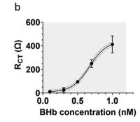
Fig. 6 Standard curve for BHb determination using BHb MIP-modified BT-Au electrode (a). (b) Shows linear range in (a) expanded. Saturation occurs at 1 nM of target protein, indicating that all MIP cavities are occupied with protein.  $K_D$  was determined to be 0.86  $\pm$  0.11 nM using the Hill-Langmuir method. Data represents mean  $\pm$  S.E.M., n = 3.
