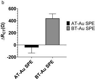
**Fig. 4** Comparison of performance of AT-Au and BT-Au SPEs, following MIP modification and protein (1 nM) rebinding. Effect on (a) CV peak anodic current change (J in  $\mu$ A mm<sup>-2</sup>) and (b) charge transfer resistance ( $R_{CT}$  in  $\Omega$ ) change. Data represents mean  $\pm$  S.E.M., n = 3.
