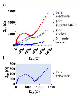
**Fig. 2** EIS Nyquist plots of ferro/ferricyanide redox marker at different stages of electrode modification (a): bare (see (b) for more detail); post E-MIP polymerisation; post template, BHb elution; and after 5 min of template, BHb rebinding.
