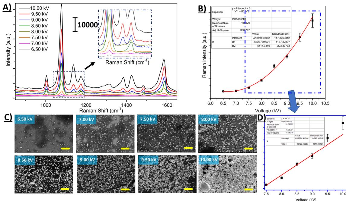
**Fig. 4** (A) SERS intensity variation for different applied voltages, (B) corresponding calibration curve and (C) SEM images for different ESI voltages as labelled. All scale bars are 500 nm. In (B) and (D) means are shown with standard deviation error bars from 10 replicates.
