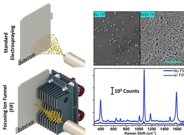
**Fig. 1** Illustration of electro spray ionisation deposition coupled with a focusing ion funnel (FIF) in comparison with standard electro spray deposition (ESD). Corresponding SEM images taken from surfaces prepared using ESD with and without a FIF are also shown, as well as representative SERS spectra acquired with 10<sup>-5</sup> M 4-ATP for both setups.
