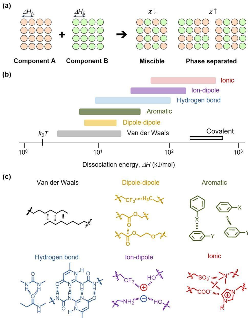
Fig. 3 Intermolecular interactions for materials design. (a) When two components are mixed, the interaction parameter  $\chi$  is a determinant factor for their miscibility. (b) A scale of the dissociation energy of diverse molecular interactions. The  $k_B T$  is thermal energy at room temperature. (c) Representative molecular moieties for different intermolecular interactions.
