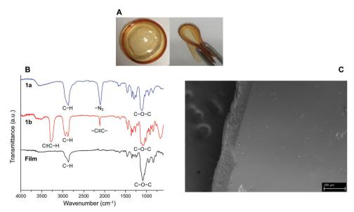
Fig. 1 (A) Digital images of obtained flexible hydrogel films (diameter of circular film = 4 cm). (B) FTIR spectra of 1a, 1b and the film. (C) SEM image of the hydrogel film. Scale bar =  $300 \mu m$
