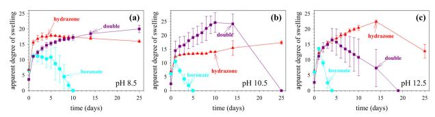
Fig. 5 Temporal evolution of the apparent aqueous degrees of swelling of the three types of hydrogels, each prepared at three different pH values, (a) 8.5, (b) 10.5 and (c) 12.5, and equilibrated in an aqueous buffer of pH the same as that at its preparation.
