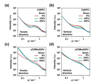
Fig. 7 SAXS profiles of C(9)PU with 0%, 100% and 200% strains in the (a) tensile and (b) vertical directions. SAXS profiles of γCDMe(9)PU with 0%, 100% and 200% strains in the (c) tensile and (d) vertical directions.
