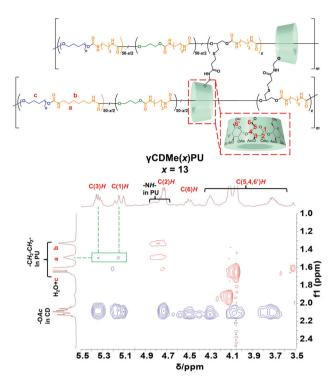
Fig. 2 600 MHz 2D NOESY NMR spectrum of γCDMe(13)PU in chloroform-d. The NOE correlation signals between the TAcγCD units and the PU main chains are highlighted.
