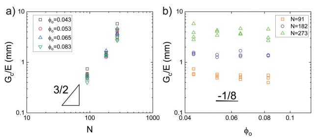
Fig. 2 Plots of the elastofracture length against (a) N and (b)  $\phi_0$  showing strong agreement with the scaling predictions of eqn (6). Data is taken from pure shear notch tests. Agreement between the data and theoretical scalings shows that altering N is a more effective means of tuning  $G_c/E$ .
