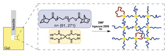
Fig. 1 Sketch showing the experimental geometry and network chemistry used in this work. This is the same synthetic approach employed recently to demonstrate a strong connection between molecular structure and both  $\it E$  and  $\it G_{c}$ . <sup>16</sup>
