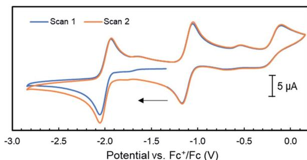
Fig. 5 Cyclic voltammograms of complex **6** (1 mM) in THF/[Bu<sub>4</sub>N]PF<sub>6</sub> (scan rate = 0.1 V s<sup>-1</sup>); the arrow indicates the scan direction.
