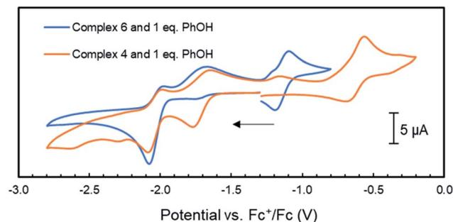
Fig. 6 Cyclic voltammograms of complex **4** and **6** (1 mM) with the addition 1 mM of phenol in THF/[Bu<sub>4</sub>N]PF<sub>6</sub> (scan rate = 0.1 V s<sup>-1</sup>); the arrow indicates the scan direction.
