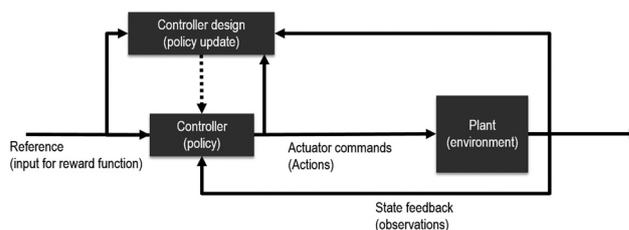
Fig. 5 Reinforcement learning can be described<sup>30</sup> as a method to tune, enhance or substitute traditional control systems.
