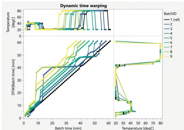
**Fig. 22** A comparison between the (original) batch time vs. time dynamically warped shows the rate at which the batches are progressing relative to the reference (batchID 1). In this illustrative example, batches are getting shorter so the rate is always positive.
