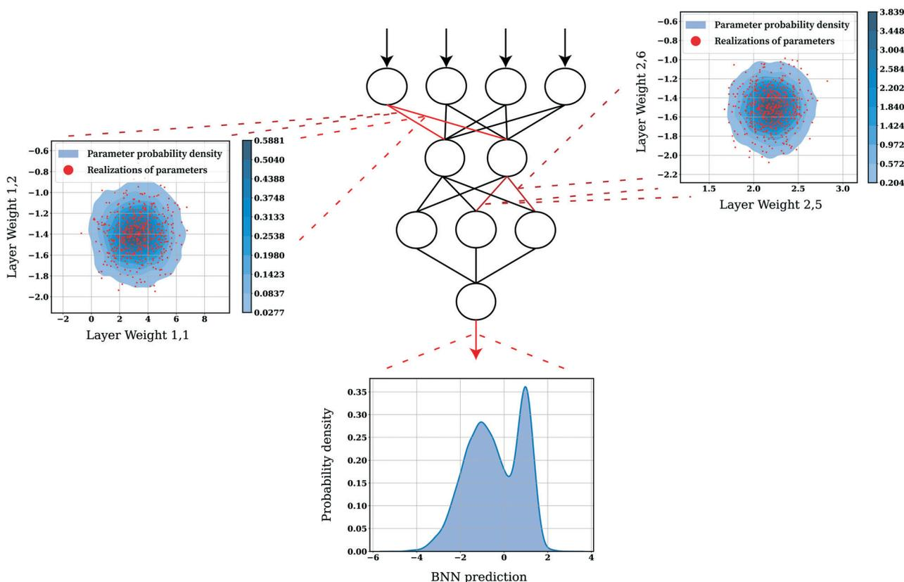
**Fig. 27** Figurative description of the Bayesian approach to express modeling uncertainty in neural networks. The top two subplots show the covariance between two-parameter distributions in the first and second layers of the network, respectively. The bottom subplot demonstrates the generation of a predictive distribution by Monte Carlo sampling the parametric distributions identified *via* approximate Bayesian inference.
