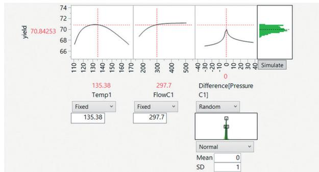
**Fig. 24** Propagation of input-output uncertainties. The lack of control in pressure is simulated by including a random normal distribution in the predictive model input, generating a distribution of yield (output).
