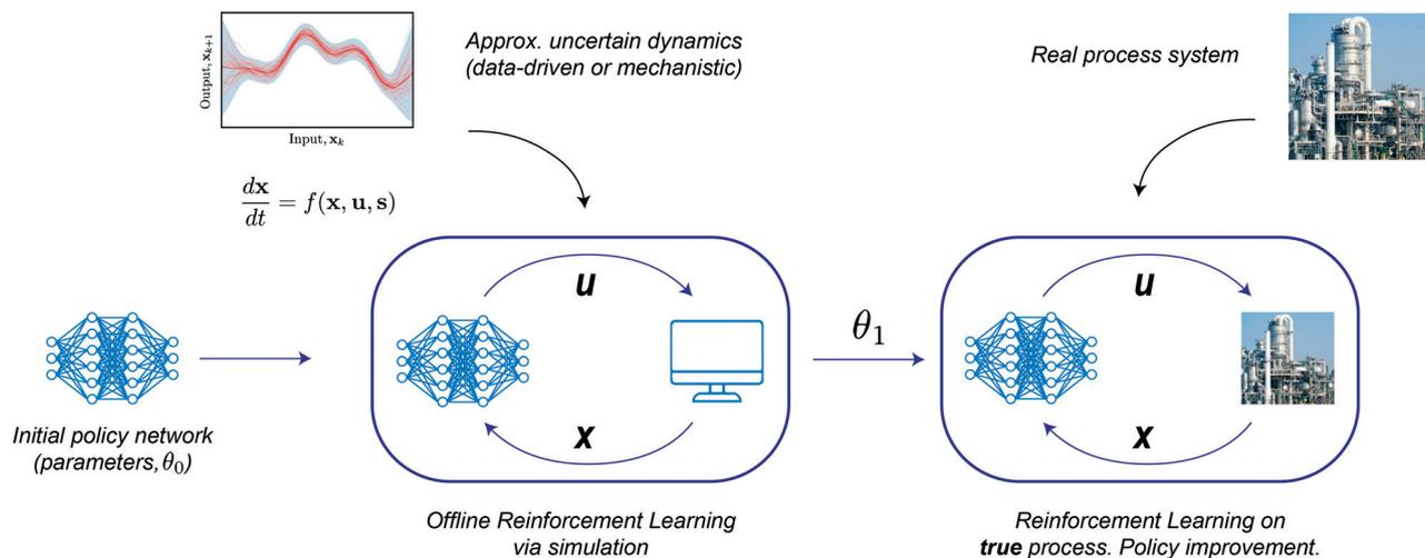
**Fig. 35** A schematic representation of a framework for the application of RL to chemical process optimization. Initial policy learning is first conducted offline *via* simulation of an approximate process model. The policy is then transferred to the real system where it may be improved either *via* iterative improvement of the offline model or directly from the data accrued from process operation.
