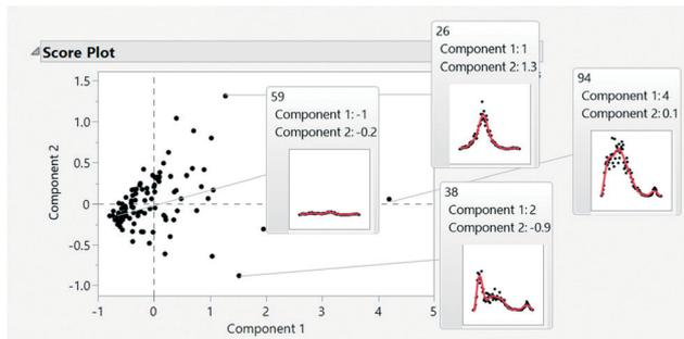
**Fig. 20** Functional PCA summarizes the batch information into new coordinate variables that capture variability seen during the batch. In the image, batch curves can be described again using a combination of components 1 and 2.
