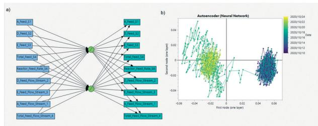
**Fig. 13** Similar to PCA, autoencoders are neural networks (a) that reduce the dimensionality of the data by restricting the number of nodes in the middle layers. The transition between two feeding steady-state regimes for a Tennessee Eastman process (simulated data<sup>49,50</sup>) is captured (b) while noisy and redundant measures are discarded.
