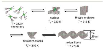
Fig. 3 Schematic assembly mechanism for the formation of helical fibrous aggregates Agg. II<sub>L</sub> of dye 1 upon slow cooling from 343 K to 273 K in the chiral limonene solvent.
