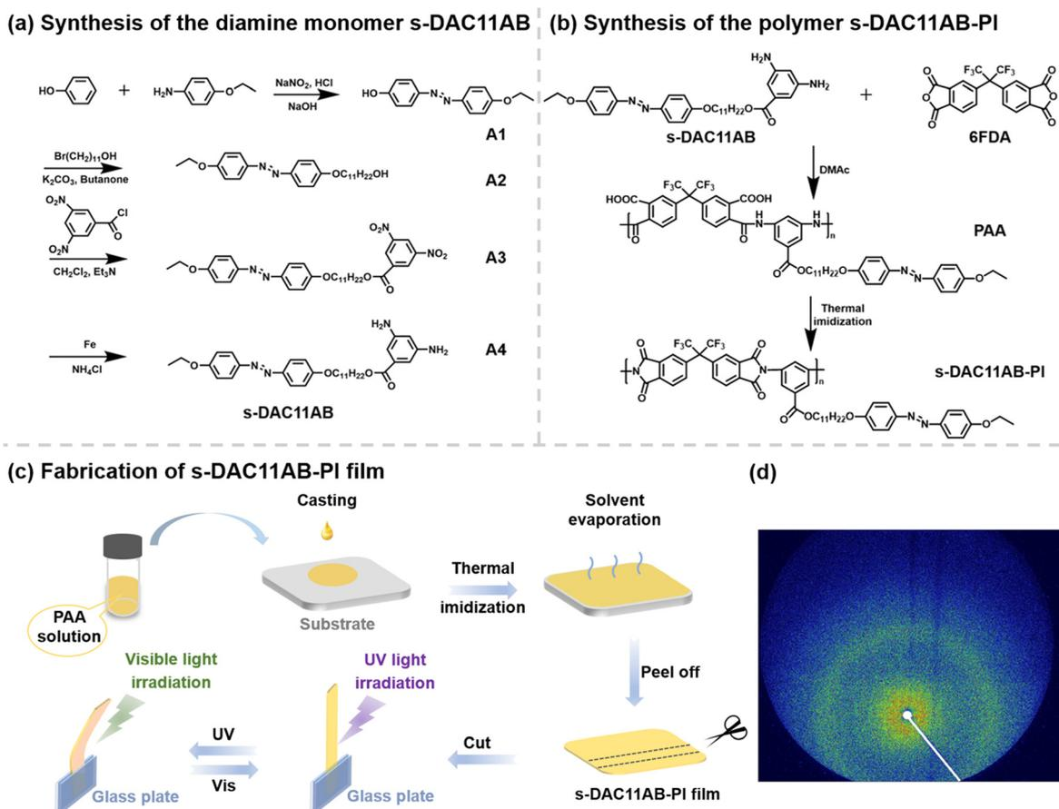
**Fig. 1** (a) The synthesis route and chemical structure of s-DAC11AB. (b) The synthesis route and chemical structure of s-DAC11AB-PI. (c) Schematic diagram showing the fabrication and photoinduced deformation of the s-DAC11AB-PI film. (d) The 2D WAXD pattern of the s-DAC11AB-PI film showing the isotropic amorphous structure of the film.
