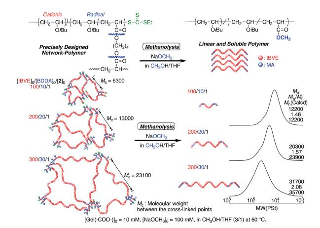
Fig. 2 SEC curves of the products after methanolysis of the cross-linked polymer gel prepared in the same experiments as in Fig. 1.
