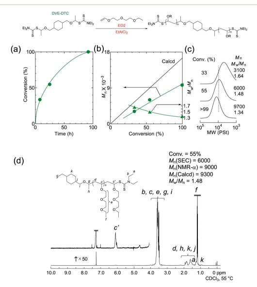
Fig. 3 Living cationic polymerization of EO2 with bifunctional dithiocarbamate (DVE-DTC):  $[EO2]_0/[DVE-DTC]_0/[EtAlCl_2]_0/[THF]_0 = 1000/10/15/400$  mM in toluene at 0 °C. (a) time-conversion, (b)  $M_n$  and  $M_w/M_n$  curves, (c) SEC curves, and (d) <sup>1</sup>H NMR spectrum of the obtained polymer.
