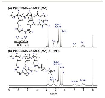
Fig. 2  $^{1}\text{H}$  NMR spectra of (a) P(OEGMA-co-MEO $_{2}\text{MA})$  and (b) P(OEGMA-co-MEO $_{2}\text{MA})$ -b-PMPC.
