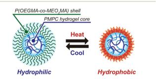
Fig. 8 Schematic illustration of the morphology of PMPC core-shell microgels and their temperature-responsive behaviour.
