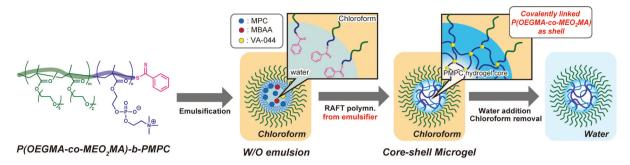
Fig. 1 Schematic illustration of the preparation of PMPC core-shell microgels by inverse miniemulsion RAFT copolymerization of MPC and MBAA using water-soluble P(OEGMA-co-MEO<sub>2</sub>MA)-b-PMPC emulsifier.
