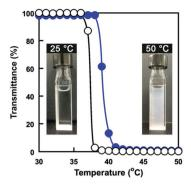
Fig. 7 Changes in transmittance (650 nm) of a PMPC core-shell microgel dispersion in water (●) and an aqueous P(OEGMA-co-MEO<sub>2</sub>MA) solution (O) as a function of temperature. (Inserted photos: PMPC coreshell microgel dispersion at 25 °C and 50 °C.)
