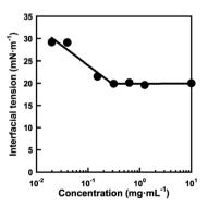
Fig. 4 Effect of P(OEGMA-co-MEO<sub>2</sub>MA)-b-PMPC concentration on the interfacial tension of a water-chloroform interface at 25 °C. The interfacial tension was measured using the pendant drop technique with a contact angle meter.
