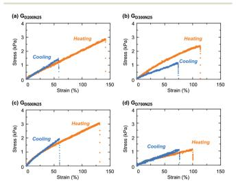
Fig. 4 Uniaxial tensile tests of the gels with a CD structure in heating and cooling states prepared from various macro-CTAs with different molecular weights: (a)  $G_{D200N25}$ , (b)  $G_{D300N25}$ , (c)  $G_{D500N25}$ , and (d) G<sub>D700N25</sub>.
