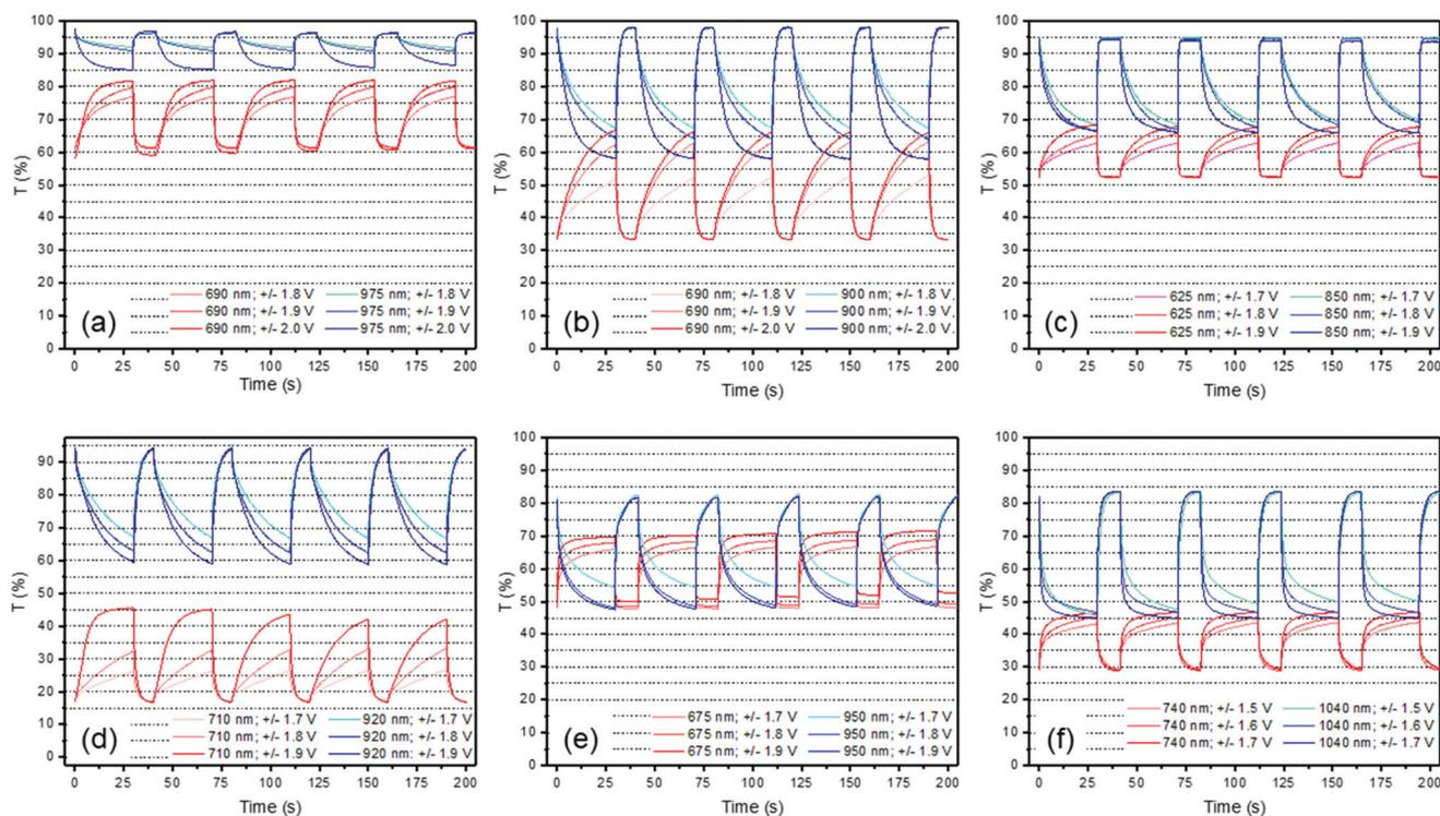
Fig. 3 Square-wave potential step absorptiometry of ECDs containing polymers (a) **p(IID-T)**, (b) **p(IID-2T)**, (c) **p(IID-3T)**, (d) **p(IID-TT)**, (e) **p(IID-EDOT)** and (f) **p(IID-2EDOT)** undergoing five cycles of EC switching at different voltages at 30 s/10 s oxidation/reduction intervals.
