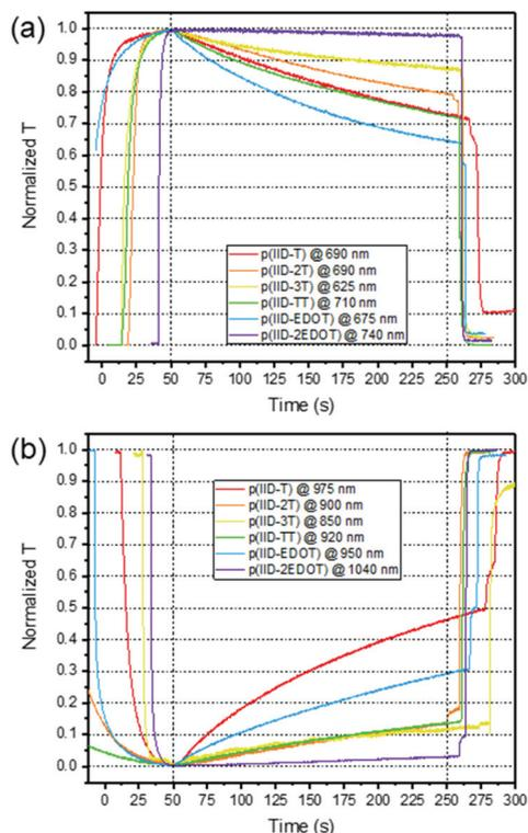
**Fig. 4** Optical memory retention of the six polymers at their respective visible/far-red (a) and NIR (b) wavelengths-of-interest as reflected by the changes in normalized transmittance ( $T$ ) after oxidation, under open-circuit conditions over 200 s. The vertical dotted lines in both graphs at time = 50 s and 250 s indicate the time points where the ECDs were fully charged (oxidised) and subjected to open-circuit conditions and after 200 s.
