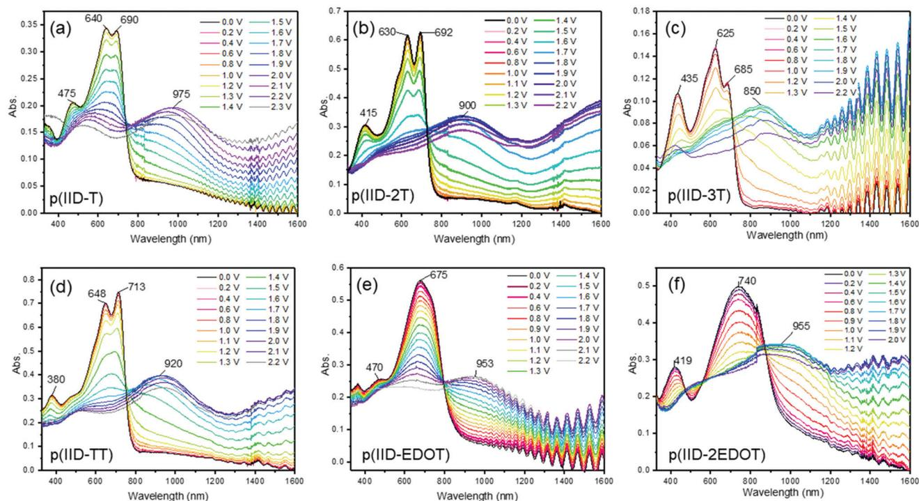
Fig. 1 Spectroelectrochemistry of isoindigo polymers (a) **p(IID-T)**, (b) **p(IID-2T)**, (c) **p(IID-3T)**, (d) **p(IID-TT)**, (e) **p(IID-EDOT)** and (f) **p(IID-2EDOT)** in fabricated ECDs, undergoing electrochemical oxidative doping.
