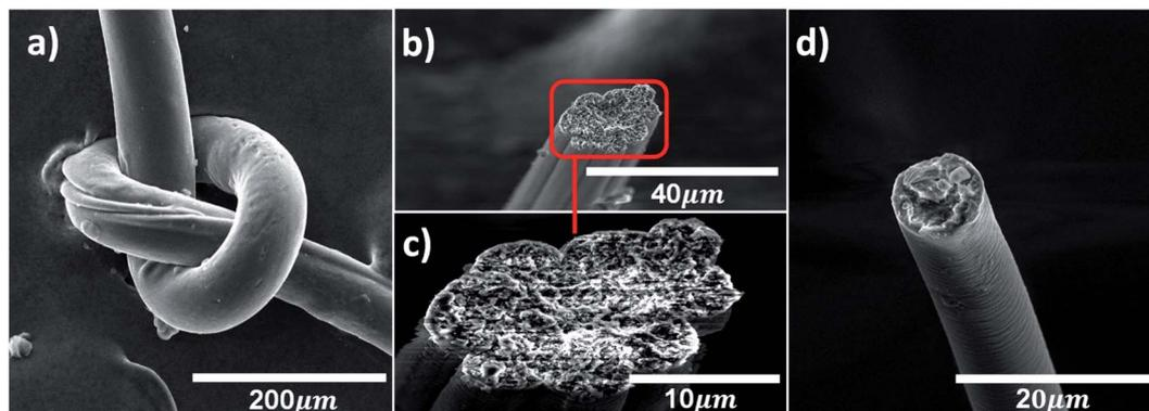
Fig. 3 SEM images of BNNTs/PVA fibers produced from dispersions containing 5 mass% PVA in an EtOH coagulation bath. (a) A fiber obtained from a dispersion of 0.1 mass% pristine BNNTs showing the mechanical robustness (knot). The scale bar is 200  $\mu\text{m}$ . The cross-section of fibers obtained from dispersions containing (b and c) 0.1 mass% pristine BNNTs and (d) 0.1 mass% purified BNNTs. The scale bars are 10, 20, and 40  $\mu\text{m}$ , respectively.
