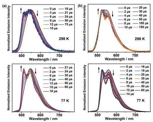
Normalized time-resolved emission spectra of (a) 1 and (b) 4 doped at 5 wt% in MCP at 298 K and 77 K.
