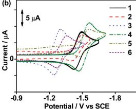
Fig. 1 Cyclic voltammograms for (a) oxidative and (b) reductive scans of **1–6** in degassed dichloromethane (0.1 M  $^{n}$ Bu<sub>4</sub>NPF<sub>6</sub>) at 298 K.
