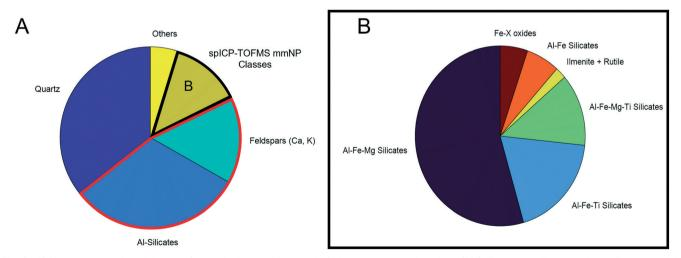
Fig. 6 A) Mass percent of particle types/minerals detected in sample S1 by automated mineralogy (AM). The red outlined section indicates particle types that would have likely been detected as Al single metal particles (smNPs) by spICP-TOFMS due to the inability to accurately quantify the other constituents (Si, Ca, K, and Na). B) Mass percent of mineral types that overlapped in elemental composition with multi metal nanoparticle (mmNP) groups observed by spICP-TOFMS.
