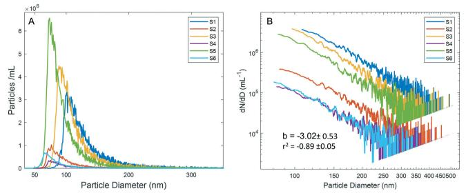
Fig. 2 A) Particle size distributions for <sup>27</sup>Al obtained by spICP-QMS. B) Reprocessed PSD data, with data normalized to number per nm (dN/dD) versus diameter and plotted in log space. The slope (b) and  $r^2$  are an average of all samples; +/-1 SD.
