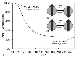
Fig. 2 (i) para- and (ii) ortho-hydrogen spin isomers. (iii) para-Hydrogen content of hydrogen at equilibrium as a function of temperature.
