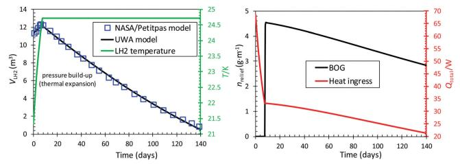
Fig. 16 Change of liquid hydrogen stored volume and boil-off gas rate over time in a 12.5 m<sup>3</sup> storage tank. Symbols correspond to the literature values while solid curves correspond to the value calculated using the model developed at the University of Western Australia (UWA).
