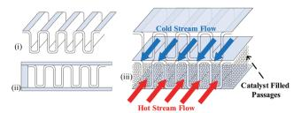
Fig. 12 Illustration of the (i) fins, (ii) empty channels and (iii) catalyst-filled channels in a plate-fin heat exchanger with cold and warm streams flowing through.
