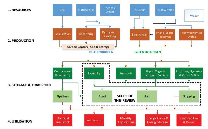
Fig. 1 The hydrogen value chain and its relation to the focus of this review into hydrogen liquefaction.
