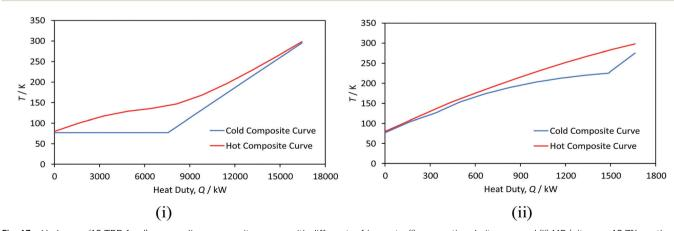
Fig. 13 Hydrogen (10 TPD feed) pre-cooling composite curves with different refrigerants: (i) conventional nitrogen and (ii) MR (nitrogen 18.7%, methane 26.4%, ethane 20.3%, propane 16.9%, i-butane 17.8%) using the PRICO system. Hydrogen feed condition: T = 298.15 K, p = 3 MPa. Hydrogen intermediate condition: T = 80 K, p = 3 MPa. Minimum temperature approach of heat exchanger = 3 K.
