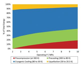
Fig. 5 Distribution of exergy requirements for each stage of hydrogen liquefaction based on operating pressure.
