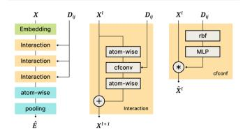
Fig. 3 A schematic depiction of the SchNet architecture with its subunits. The left column shows an overview, and middle and right columns detail the Interaction and cfconf blocks. X is an atom's representation.  $D_{ii}$  is the pairwise distance matrix. Atom-wise blocks are multilayer perceptrons applied to each atom representation independently
