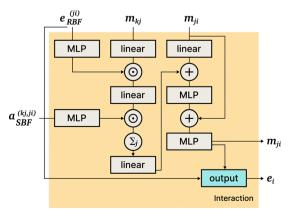
Fig. 5 DimeNet+ + architecture: the Interaction block
