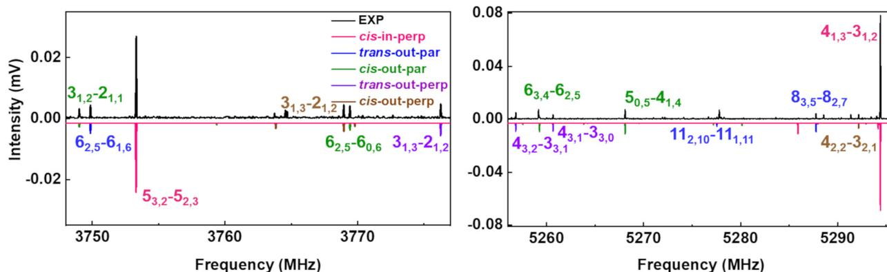
**Fig. 3** Parts of the 2–8 GHz rotational spectrum of AMPA with the labelling scheme of the rotational transitions as  $J'_{K'_a K'_c} \leftarrow J''_{K''_a K''_c}$ . The top part shows the experimental spectrum and the bottom part represents the simulations using the fitted rotational parameters for AMPA conformers (Table 2). The relative intensities are based on the predicted dipole moment components (Table 1).
