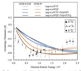
Fig. 7 Comparison of the  $\beta(\varepsilon)$  profiles for photodetachment into the  $X^3\Sigma^{-1}$ state of SO obtained using EOM-EA/SF (different shades of blue) and EOM-IP (different shades of orange) Dyson orbitals with different basis sets. Symbols represent the experimental data reproduced from Fig. 2(a) for comparison.
