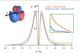
Fig. 4 A plot of  $y \cdot \phi^{d}(y)$  versus  $\hat{y}$  for Dyson orbitals computed for detachment from SO<sup>-</sup>( $X^2\Pi$ ) to the  $X^3\Sigma^-$  state of SO. The figure shows Dyson orbitals computed using CCSD → EOM-IP-CCSD (orange) and EOM-EA- $CCSD \rightarrow EOM-SF-CCSD$  (blue) wave functions with the aug-ccpVTZ+5s5p5d5f basis set. The y axis was chosen for this plot, because it goes through a region of the Dyson orbital that has a large electron density
