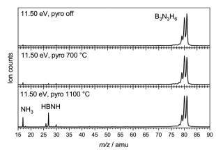
Fig. 1 Mass spectra of borazine at different pyrolysis powers, corresponding to estimated temperatures of 700 °C (30 W) and 1100 °C (60 W).
