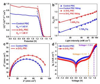
Fig. 3 (a) C-V curves, (b) dependence of  $V_{\rm oc}$  on light intensity, (c) EIS spectra, and (d) dark J-V curves of control and  $ZrO_2$ -capped CsPblBr<sub>2</sub> PSCs.
