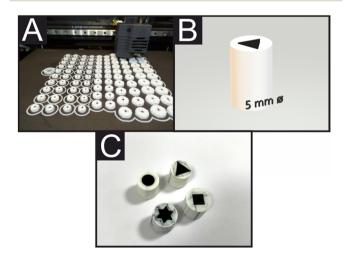
Fig. 1 (A) Photograph of FFF printing of the AM electrodes, showcasing the ability of printing 100 electrodes at the same time, with different shapes and/or dimensions (B) CAD view of a 5 mm equilateral triangle electrode. (C) Overview comparison of the 7.5 mm disc, square, equilateral triangle and (6 point) star electrodes shapes.
