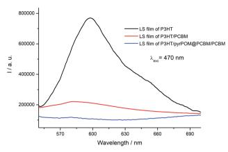
**Fig. 6** Fluorescence quenching of the thin film of P3HT emission when transferred on ITO substrate (black line), on ITO/**PCBM** LS film (red line) and on ITO/**PCBM/pyrPOM@PCBM**/P3HT stacking (blue line). Excitation wavelength: 470 nm.
