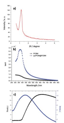
Fig. 4 (a) XRD measurement shows a periodicity of (7.6  $\pm$  0.2) nm of the LS pyrPOM@PCBM layer. (b and c) The dielectric loss of pyrPOM@PCBM, dramatically different from that one of PCBM, suggests that an electric dipole is created at the opposite edges of the nanodomains. Increasing the frequency, the dielectric permittivity of pyrPOM@PCBM LS film becomes negligible.
