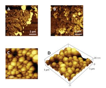
Fig. 3 Topography of PCBM (A) and pyrPOM@PCBM LS film (deposited by one run, B), (C) A magnification of the globular domains evidences that the size of the aggregates is comprised between 100 and 300 nm. (D) Three-dimensional topography suggests that the aggregates are about 20 nm high
