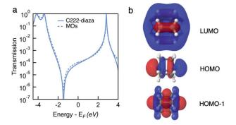
Fig. 4 (a) Transmission functions of C222-diaza, calculated as  $T(E) = |t_{\rm LUMO} + t_{\rm HOMO} + t_{\rm HOMO-1}|^2$  (dashed line) overlaid with Landauer transmission in the wide-band limit (solid). (b) MOs of C222-diaza calculated using DFT with B3LYP functional. White, black and blue atoms represent H, C and N, respectively.
