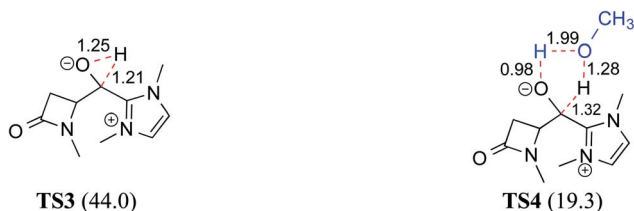
Fig. 1 The key geometric features of 1,2-direct proton transfer and methanol assisted proton transfer transition states for the formation of the Breslow intermediate. The activation barriers ( \Delta G^\ddagger in kcal mol -1 ) at the PCM (DCM) /B3LYP/6-31G** level of theory are given in parentheses. Distances are in angstroms.
