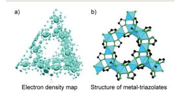
Fig. 9 Charge-flipping method is applied to analyze the electron density map of metal-triazolates (a) represented in the form of structural connectivity (b). Reproduced with permission.<sup>84</sup> Copyright 2012, Wiley-VCH.
