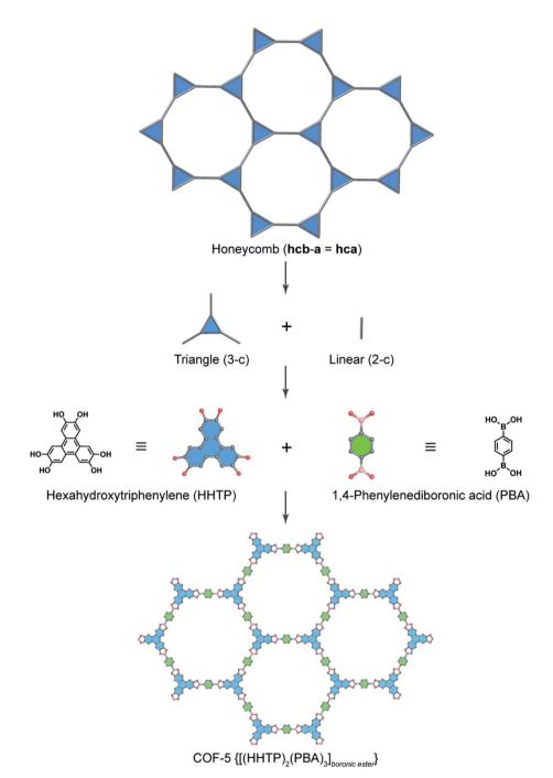
Fig. 2 Reticular design of honeycomb topology. Deconstruction of the augmented net of honeycomb (hcb-a, also termed hca) into triangular (3-c) and linear (2-c) units which correspond to hexahydrotriphenylene (HHTP) and 1,4-phenylenediboronic acid (PBA), respectively. HHTP and PBA are reticulated into the 2D structure of COF-5 [(HHTP)<sub>2</sub>(PBA)<sub>3</sub>]<sub>boronic ester</sub> adopting boronic ester linkages.
