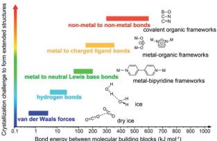
Fig. 1 Schematic diagram of the stability and crystallization problem of COFs compared to other extended structures and molecular compounds. Reproduced with permission. Copyright 2016, American Chemical Society.
