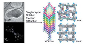
Fig. 6 Single-crystal structure analysis of COF-320 using the RED technique. COF-320 crystallized in single sub-μm crystals (top left) and was the first sample for which RED data were collected and reconstructed to the 3D reciprocal lattice (bottom left). Right side shows the crystal structure of the 9-fold interpenetrated dia framework solved at 89 K and 298 K. Reproduced with permission.<sup>62</sup> Copyright 2013, American Chemical Society.
