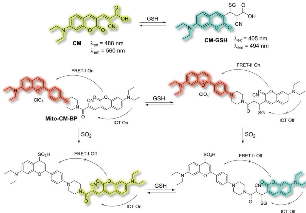
Scheme 28 ICT and FRET-based probe **Mito-CM-BP** developed to allow for the simultaneous detection of GSH and  $\text{SO}_2$ .
