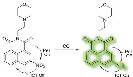
Scheme 29 A lysosome targetable fluorescent probe **LysoFP-NO<sub>2</sub>** for detection of CO.
