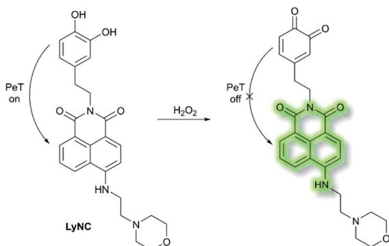
Scheme 18 The recognition mechanism of probe **LyNC** towards H<sub>2</sub>O<sub>2</sub>.
