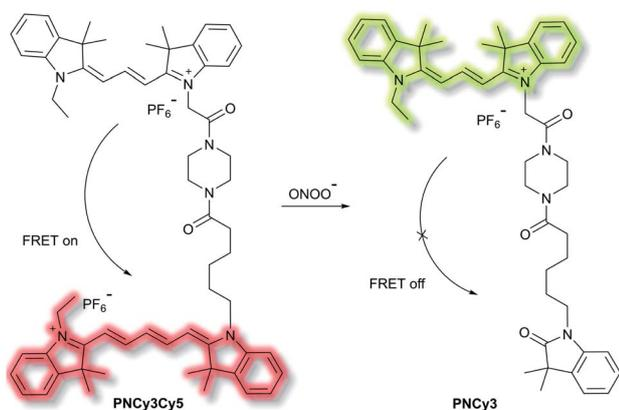
Scheme 3 Cy3 and Cy5 (energy donor and acceptor)-based FRET fluorescent probe PNCy3Cy5, developed for the ratiometric detection of  $\text{ONOO}^-$ . Also shown is the structure of its cleavage product PNCy3.
