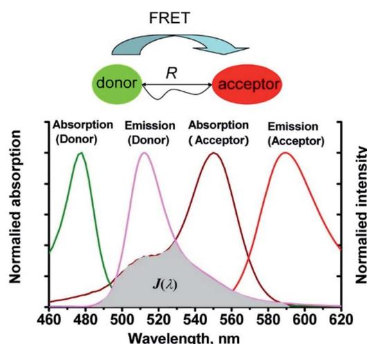
Fig. 1 The mechanism of Förster resonance energy transfer (FRET).  $R$  is the distance between the energy donor and acceptor,  $J(\lambda)$  represents the degree of spectroscopic overlap between the donor emission and the acceptor absorption. Reproduced with permission from ref. 37. Copyright 2013, American Chemical Society.
