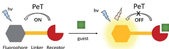
Scheme 14 The mechanism of PeT-based fluorescent probes.
