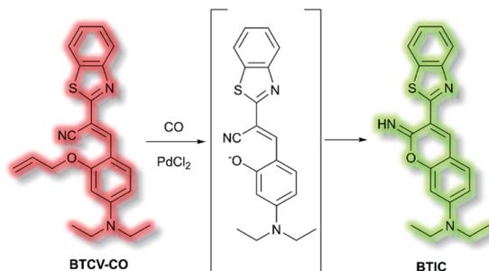
Scheme 25 Detection of CO by AIEgen BTCV-CO.
