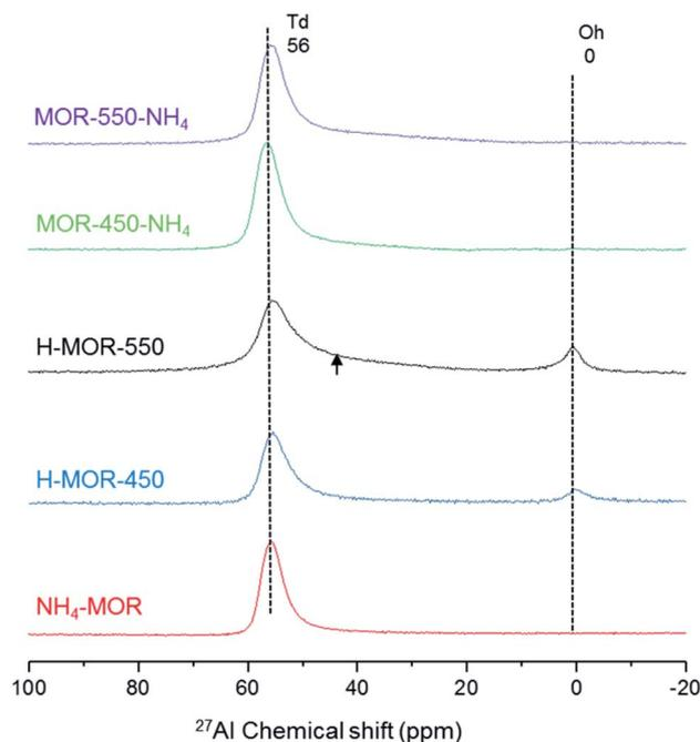
Fig. 2 <sup>27</sup>Al MAS NMR spectra of zeolite MOR under ambient conditions of NH<sub>4</sub>–MOR, H–MOR-450, H–MOR-550, MOR-450–NH<sub>4</sub> and MOR-550–NH<sub>4</sub>. The broad shoulder at the high field side of the peak corresponding to tetrahedrally coordinated framework aluminum in H–MOR-550 is highlighted by the black arrow mark.
