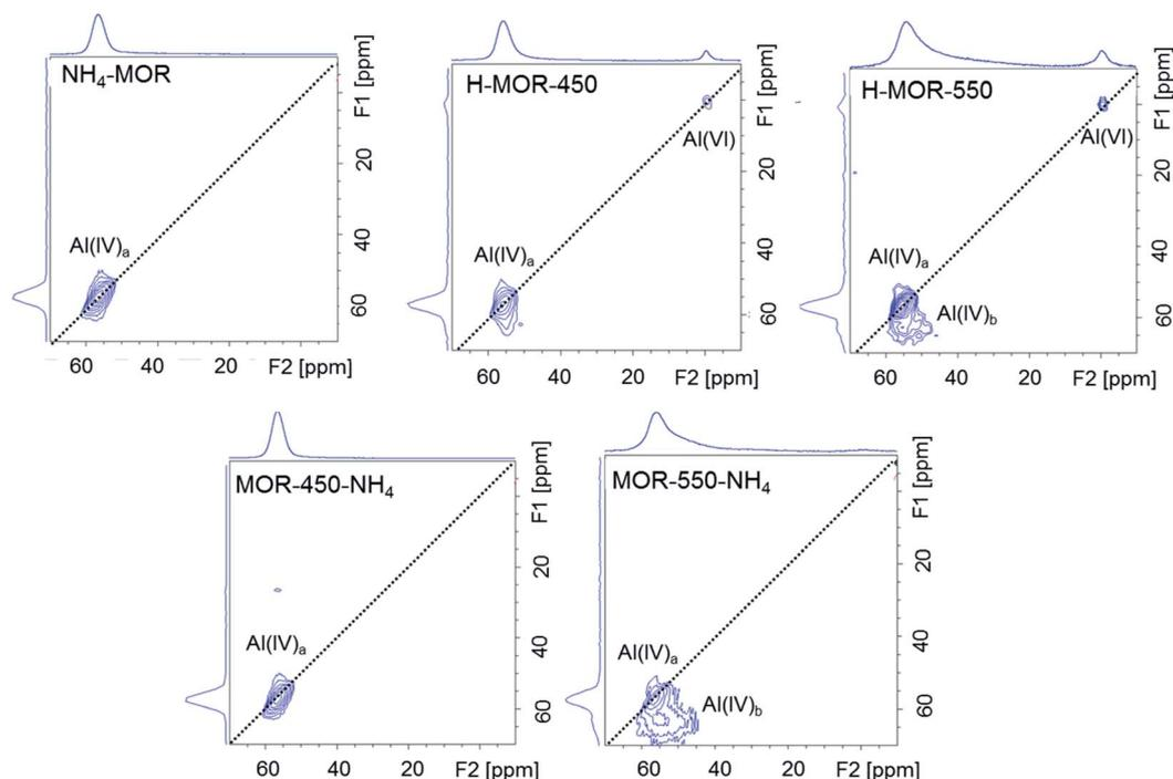
**Fig. 3** <sup>27</sup>Al MQMAS NMR spectra measured under ambient conditions for NH<sub>4</sub>-MOR, H-MOR-450, H-MOR-550, MOR-450-NH<sub>4</sub> and MOR-550-NH<sub>4</sub>. The F1 projection shows a purely isotropic dimension and the F2 projection depicts the corresponding <sup>27</sup>Al MAS NMR spectrum, which is acquired in a separate experiment.
