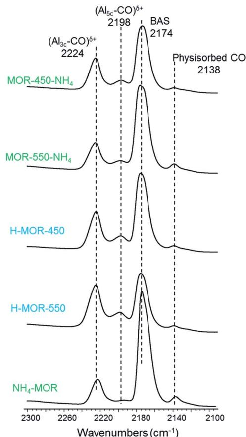
Fig. 5 FTIR spectra of adsorbed carbon monoxide over activated parent ammonium form  $\text{NH}_4\text{-MOR}$ ,  $\text{H-MOR-450}$ ,  $\text{H-MOR-550}$ ,  $\text{MOR-450-NH}_4$  and  $\text{MOR-550-NH}_4$ . The names of the samples refer to the form of the zeolite prior to heat treatment in the IR setup.
