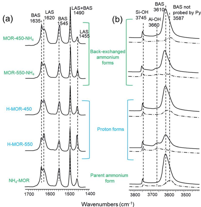
Fig. 4 FTIR spectra of (a) adsorbed pyridine over activated NH<sub>4</sub>-MOR, H-MOR-450, H-MOR-550, MOR-450-NH<sub>4</sub> and MOR-550-NH<sub>4</sub>; (b) samples activated under vacuum at 450 °C for 4 h (solid line) and after pyridine adsorption–desorption at 150 °C (dashed line) in the OH stretching region. The names of the samples refer to the form of the zeolite prior to heat treatment in the IR setup.
