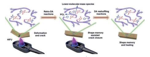
Fig. 10 A schematic diagram of the healing of a PCL-based PU with DA linkage assisted by HIFU-triggered shape memory. Copyright 2014. Reproduced with permission from Royal Society of Chemistry.
