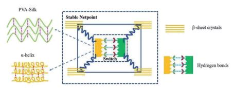
Fig. 7 Structure model of the shape memory PVA/silk hybrid.<sup>74</sup> Copyright 2019. Reproduced with permission from Elsevier.
