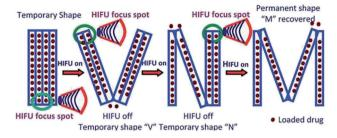
Fig. 6 Schematic illustration of the HIFU-enabled shape memory process and drug-controlled release.<sup>68</sup> Copyright 2012. Reproduced with permission from Royal Society of Chemistry.
