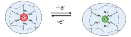
Fig. 12 Mechanism of shape memory effect and rapid reversible actuation of hydrogels with electrochemically controlled local metal ion coordination and crosslinking.<sup>123</sup> Copyright 2020. Reproduced with permission from Royal Society of Chemistry.
