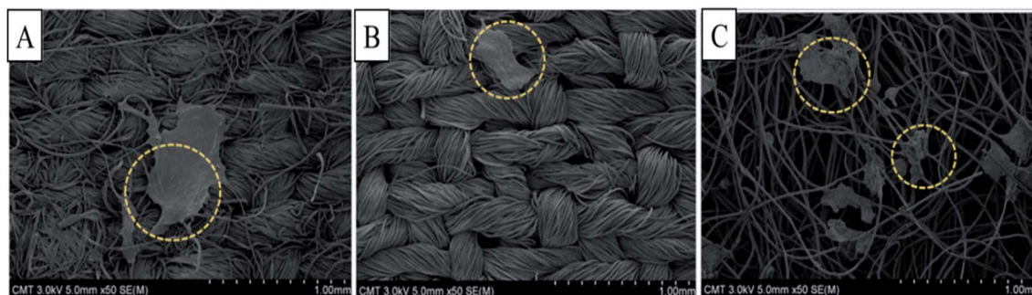
Fig. 9 SEM images of fabrics incorporated with Chinese herb microcapsule: (A) cotton; (B) polyester; (C) nonwoven; this figure is reproduced from the ref. 120 (Gigvvy science open access publishing platform, subject to CC BY-SA 4.0 creative common attribution license).
