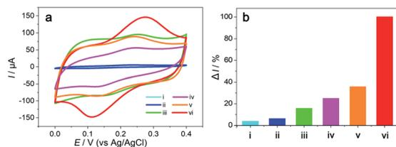
Fig. 5 (a) CVs obtained for different electrodes in 0.10 M PBS with 0.1 mM DA at a scan rate of 100 mV s<sup>-1</sup>. (b) Comparison of CVs relative response signal obtained from each electrode. (i) GCE, (ii) Hemin-doped-HKUST-1/GCE (iii) rGO/GCE, (vi) Hemin/rGO/GCE, (v) HKUST-1/rGO/GCE and (vi) Hemin-doped-HKUST-1/rGO/GCE.
