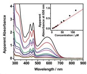
Fig. 2 Concentration-dependent UV-vis absorption spectra of complex **1** in DMSO solution in the concentration range of  $4.59 \times 10^{-6}$  to  $1.15 \times 10^{-4}$  M. Inset: A plot of apparent absorbance against concentration, monitored at 650 nm. The apparent absorbance values were obtained by correcting to 1 cm path length equivalence.
