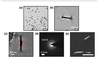
Fig. 4 TEM images of complex 3 prepared from a DMSO solution with (a) lower magnification and (b) higher magnification. (c) A TEM image of complex 3 prepared from a DMSO solution with a red circle indicating where SAED was performed and (d) the corresponding SAED pattern. (e) An SEM image of complex 3 prepared from a DMSO solution.
