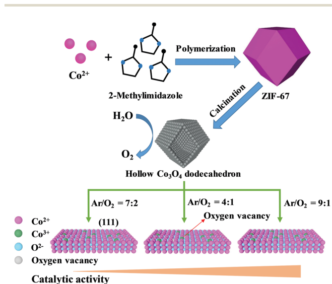
Scheme 1 Schematic of the preparation of hollow \text{Co}_3\text{O}_4 dodecahedrons and oxygen content controlled dominant exposure of the (111) facet and oxygen vacancies for the high performance OER.
