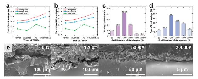
Fig. 2 (a) The open-circuit voltage ( $V_{\rm OC}$ ) and (b) short-circuit current ( $I_{\rm SC}$ ) of the four types of TENGs. (c) The measured thickness of the air-gap and (d)  $V_{\rm OC}$  with various grit numbers of commercial sandpapers. (e) The scanning electron microscope (SEM) images for the cross-section showing an air-gap between the dielectric layer and metal layer with various grit numbers of commercial sandpapers ranging from 600#, 1200#, 5000#, and 20 000#.
