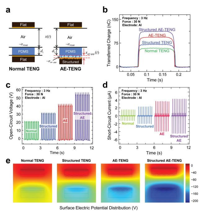
Fig. 4 (a) Schematic diagram describing the theoretical modeling for normal TENG and AE-TENG. (b) The amount of transferred charges (Q<sub>tr</sub>), (c) open-circuit voltage ( $V_{OC}$ ), and (d) short-circuit current ( $I_{SC}$ ) of the four types of TENGs at a vibration frequency of 3 Hz and an applied force of 30 N. (e) The visualization of the electric potential distribution of the four types of TENGs simulated by using a simulation software.
