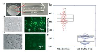
Fig. 8 (A) Picture of one blood-vessel-mimicking chip and its close-up photo; (B) optical micrograph and fluorescence image of the integrin tension sensors without inhibitor (Y-27632) treatment; (C) optical micrograph and fluorescence image of the integrin tension sensors with 20  $\mu\text{M}$  inhibitor (Y-27632) treatment. (D) The measured fluorescence intensity with and without inhibitor (Y-27632) treatment.
