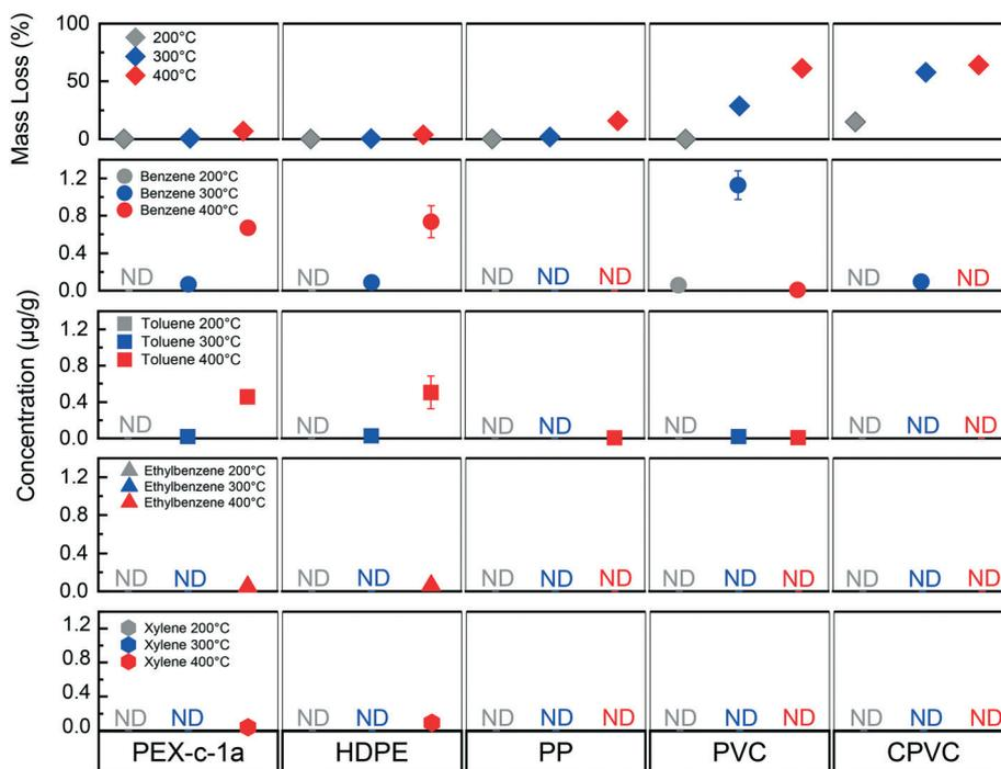
Fig. 3 Mean BTEX concentration after extracting each burned material at 200 °C, 300 °C, and 400 °C in water. The error bars reflect the standard deviation of the measurements ( $n = 3$ ). If no error bars are visible, it indicates they were smaller than the symbol size. ND indicates the compound was not detected.
