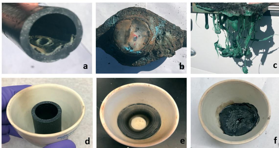
**Fig. 1** Images of fire-damaged water system components including (a) a HDPE plastic pipe, (b) a water meter, and (c) a water meter cover following the Camp Fire. Thermally degraded pipe samples in laboratory experiments include the (d) PEX-c pipe degraded at 300 °C, (e) HDPE pipe degraded at 300 °C, and (f) HDPE pipe degraded at 400 °C.
