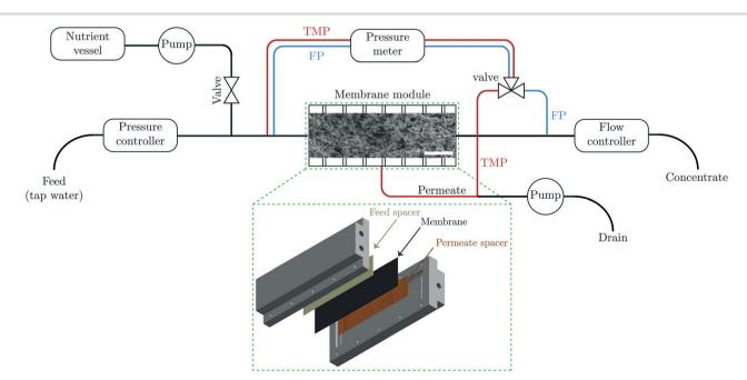
Fig. 1 Schematic illustration of the cross flow filtration set-up and SEM image of the membrane cross section (scale bar is 10 μm). TMP and FP respectively show transmembrane pressure and feed pressure lines. The insert illustrates the expanded view of the cross flow cell.
