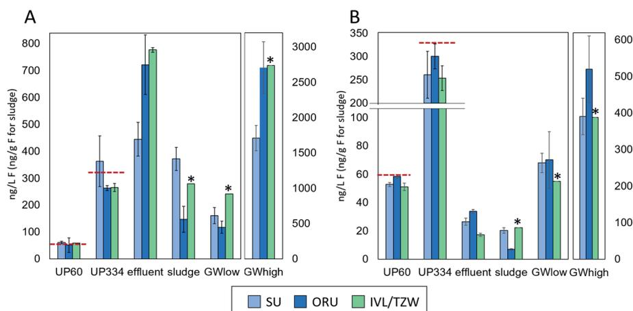
Fig. 1 Concentrations (ng L<sup>-1</sup> F for aqueous samples and ng g<sup>-1</sup> F for sludge) of EOF (A),  $\sum$ PFAS-16 (B) in interlaboratory comparison samples. Error bars represent standard deviation ( $n = 3$  for EOF and  $\sum$ PFAS-16). The dashed red lines indicate the expected concentrations. \* indicates that only a single measurement was performed.
