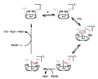
Scheme 8 Proposed mechanistic pathway for the reduction of CO<sub>2</sub> to CO by Fe-porphyrin electrocatalysts with pendant acid functionality, (OH)<sub>4</sub>.
