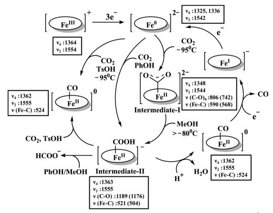
Scheme 9 Proposed mechanistic cycle for the reduction of CO<sub>2</sub> by a distal-triazole containing Fe-porphyrin. The vibrations (in cm<sup>-1</sup>) are given in the boxes.
