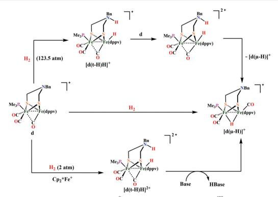
Scheme 30 Stoichiometric activation of  $H_2$  with  $[Me_3P(CO)_2Fe(N^{Bn})Fe(CO)(dppv)]$  (Fig. 30d) in the presence  $^{489}$  and absence of an external oxidant.
