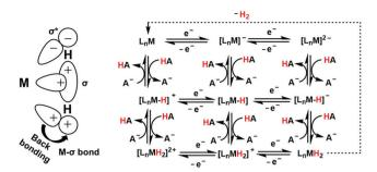
Scheme 25 Schematic presentation of the formation of M-H $_2$   $\sigma$  bond and  $M_{d\pi} \rightarrow H_2$  backdonation (left). Possible mechanistic pathways for catalytic reduction of proton to hydrogen in the natural hydrogenases or synthetic catalysts (right).
