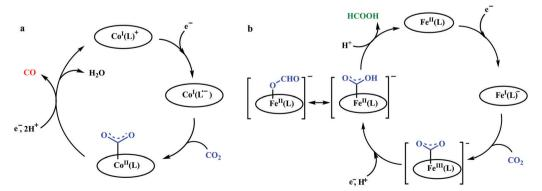
Scheme 14 Proposed mechanistic pathway for electrocatalytic CO<sub>2</sub> reduction to CO vs. formic acid; catalyzed by same ligand framework but with different metals: (a) cobalt and (b) iron
