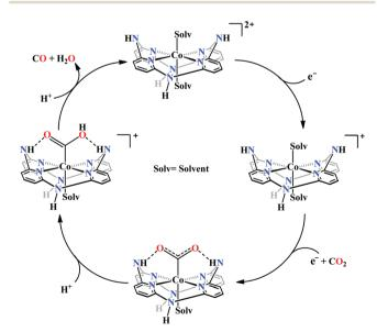
Scheme 13 Proposed mechanistic pathway for electrocatalytic CO<sub>2</sub> reduction to CO by azacalix-pyridine based macrocycles.
