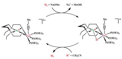
Scheme 34 Proposed mechanism of heterolytic H2 activation by complex 31a
