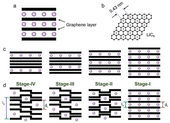
Fig. 4 Schematic illustration of (a) Li-intercalated graphite and (b) the formed LiC<sub>6</sub> structure. Two models of the stage formation process during Li<sup>+</sup> intercalation into graphite: (c) Rüdorff model and (d) Daumas-Hérold model.
