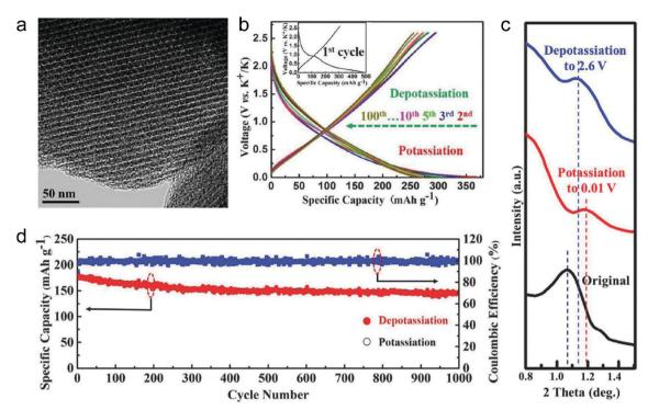
Fig. 23 (a) TEM, (b) the 2nd, 3rd, 5th, 10th, 20th, 30th, 50th, 75th, and 100th potassiation/depotassiation profiles, (c) ex situ XRD patterns, and (d) longterm cycling stability and CE of the mesoporous carbon. Reproduced from ref. 80 with permission from Wiley-VCH.
