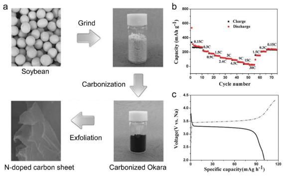
Fig. 17 (a) Schematic representation of the preparation of N-doped carbon sheets. (b) The capacity retention of the N-doped carbon sheets at current densities from 56.25 mA  $\rm g^{-1}$  to 11.25 A  $\rm g^{-1}$ . (c) Charge and discharge curves of the carbon sheets//Na<sub>3</sub>V<sub>2</sub>(PO<sub>4</sub>)<sub>3</sub> sodium ion batteries at 562 mA  $\rm g^{-1}$ . Reproduced from ref. 316 with permission from Wiley-VCH.
