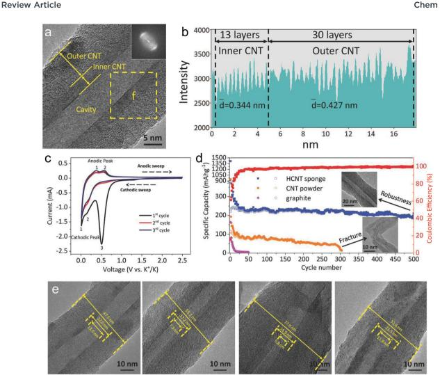
Fig. 20 (a) TEM image of a CNT. (b) Line profile obtained from the wall of a CNT. (c) CV curves of CNT sponge at  $0.3 \text{ mV s}^{-1}$ . (d) Cycling performance of CNT sponge, commercial CNT powder and graphite electrodes at a current density of 100 mA  $g^{-1}$ . (e) Ex situ TEM images of the CNT structure at different potassiation and de-potassiation potential in the first cycle. Reproduced from ref. 344 with permission from Wiley-VCH.
