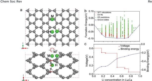
Fig. 16 (a) Structure of  $bco-C_{16}$  and the schematics of the possible Li-ion absorption sites in top and side view. (b) Formation energies predicted for the 150 different Li configurations with 5 stable intermediate phases. (c) Corresponding voltage profile (marked in red) and binding energy profile (marked in blue) calculated along the minimum energy path. Reproduced from ref. 298 with permission from United States National Academy of Sciences.
