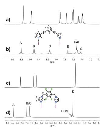
Fig. 1 Selected region of <sup>1</sup>H NMR spectra (500 MHz, CD<sub>3</sub>CN, 298 K) for ligand L1 (a), macrocycle 1 (b), the ligand L2 (c) and macrocycle 2 (d).
